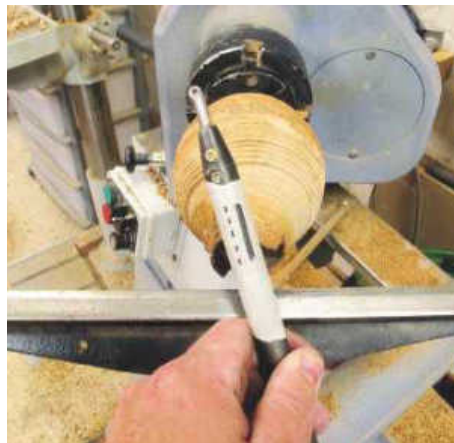
STEP 15. Trying to work out the position of the cutter while you are inside the work is never easy. The markings on the top show the cutter pointing at 12 o'clock (dotted line) and the optimum position of cutting (solid line)
